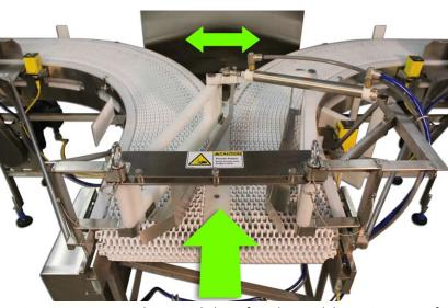
Diverging conveyor takes a single line of product and diverts in to one of two lanes for further processing. It also rotates the product 90° for the next down-line process.
