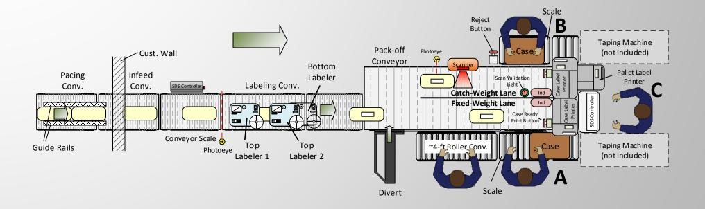
**Station A** – When a case is filled, a button would be pressed that would print a fixed-weight case label for the last 4, or 8, cheese blocks.
