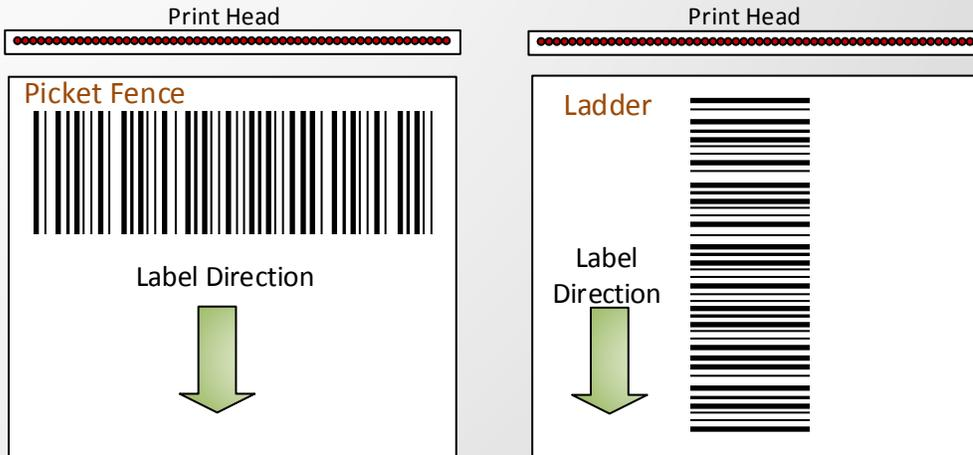
The people on the “Picket” side of the fence will argue they get a higher quality barcode because the edges of the bars are crisper due to a print head staying on for an extended period of time. Each line in the barcode requires the heaters to turn on and off once.
