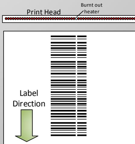
This barcode is still scannable so printing labels can continue. The ladder orientation provides some time for the line operators to eventually change out the print head.
