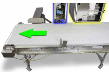
A barcode scanner (blue) verifies readability to ensure proper label placement from applicator (yellow). A divert will remove the package if the label cannot be read.
