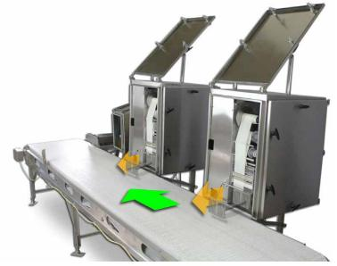
Dual printer/applicator is ideal for high capacity lines since label changeover can occur without stopping the labeling process or two different labels can be printed consecutively.
