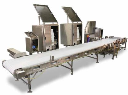
Totes can be labeled via a side-apply labeler with an additional optional backup label applicator (shown).
