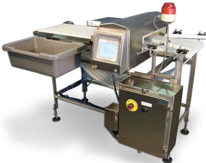
Metal detector with alarm light and divert that will reject metal containing food product into a grey bin.
