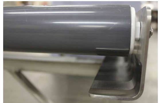
Under-bent side rails allow water to run off.
