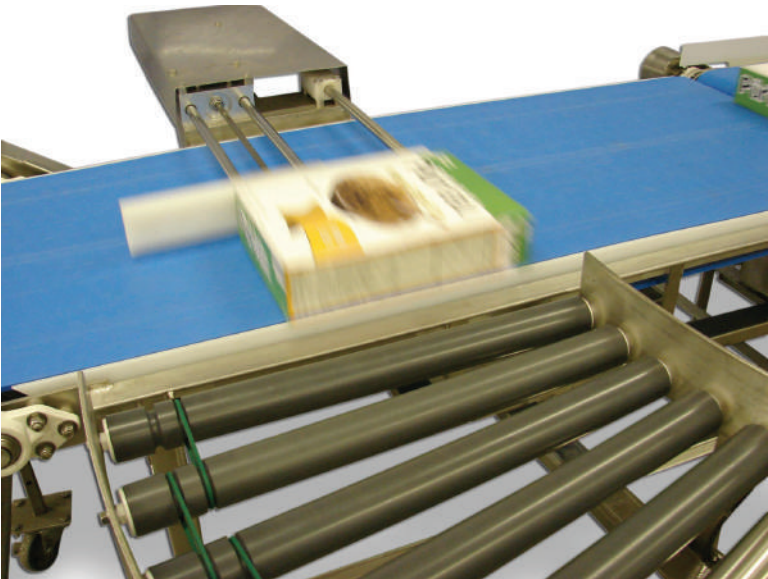
Divert Conveyors send boxes to other lines
