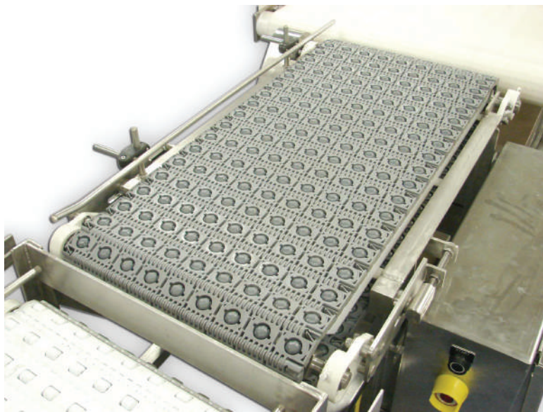
Conveyor with 30° roller activated conveyor belting moves boxes from one side of the belt to the other
