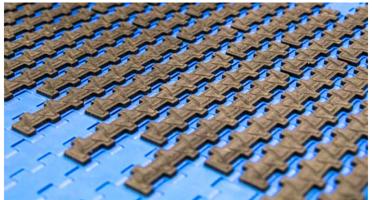
Rubberized texture of the grip belting keeps product steady through the labeling process.
