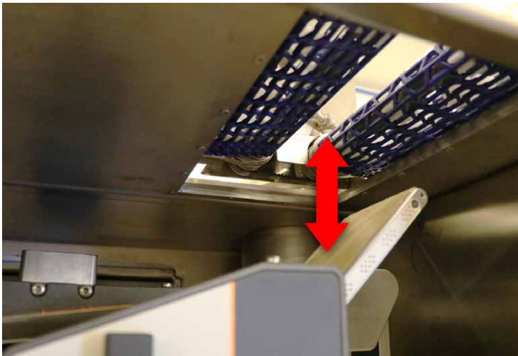
Bottom labeler raises and lowers pneumatically to store for washdown. (Cover must be secured for washdown).
