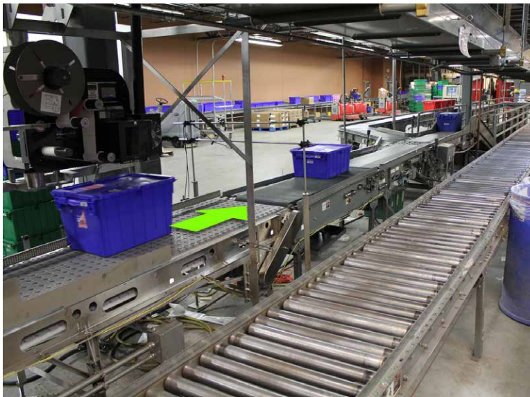
Plastic totes (of different heights) being labeled on the top. The system scans the height of the tote and adjusts the applicator arm accordingly.
