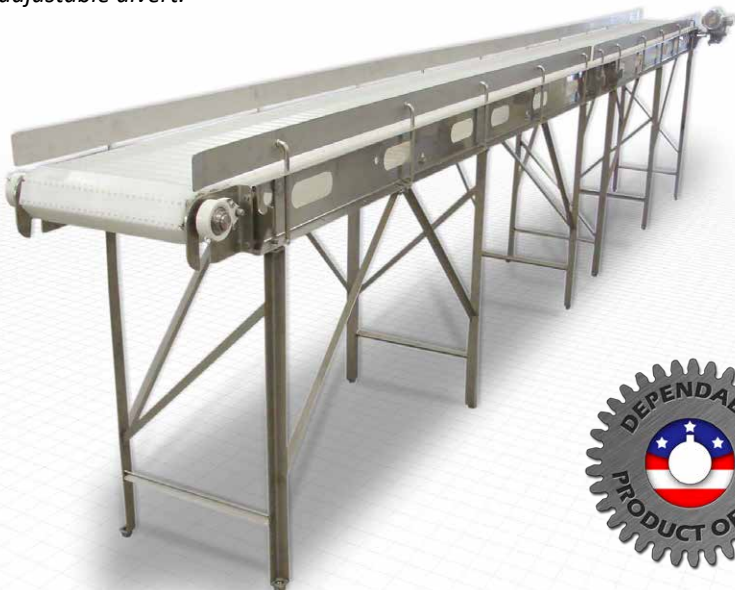
Easy-to-Clean conveyor with an open frame design. The openings along the belting frame permit access to the undersides of the belt. The cross bracing support underneath the conveyor is rotated to eliminate standing water.
