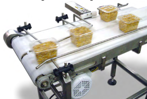
Line convergers combine multiple lines to single lines
