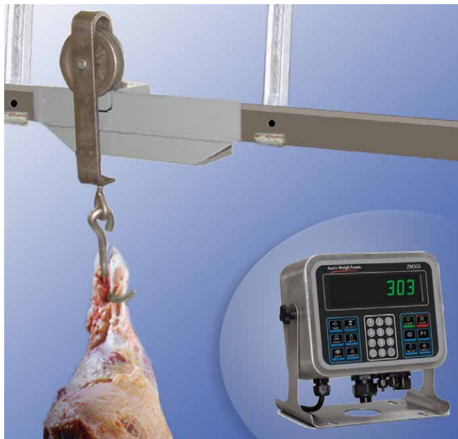
Representation of the static weighing of a carcass on our static monorail. Using the monorail with a ZM-303 indicator with keyboard allows entry of a specific trolley tare.
