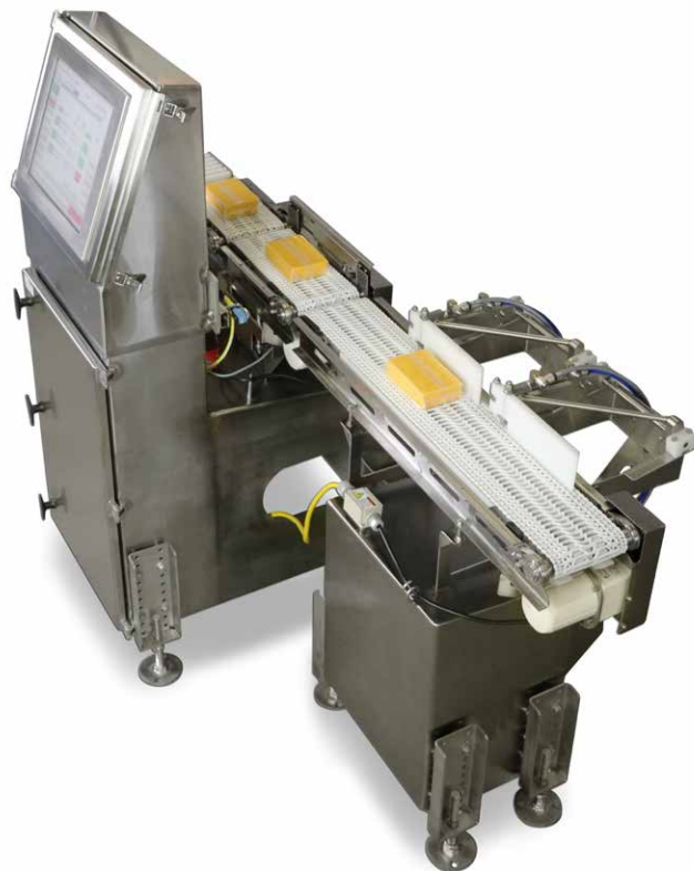
In-motion checkweigher with infeed conveyor (right), 17-inch HMI touchscreen and outfeed conveyor with divert mechanism
