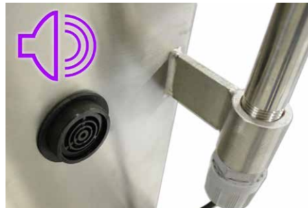
An audible alarm can be used to notify a worker of multiple rejects.
