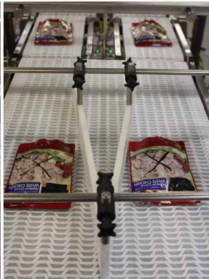
Optional product guides can be used for a variety of functions, including keeping products from tipping or aligning product for traveling squarely across the scale.
