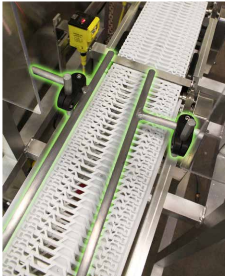
Optional product guides can be used for a variety of functions, including keeping products from tipping or aligning product for traveling squarely across the scale.
