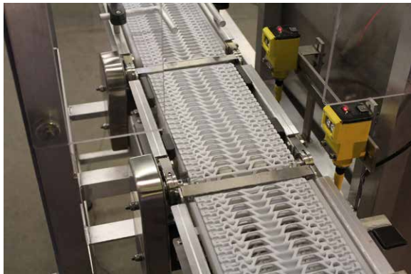
Stainless steel transition plates allow small diameter products to easily transfer without tipping.
