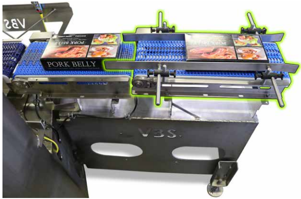
Optional pacer belt can be used to ensure products are evenly spaced thereby reducing weighing errors.
