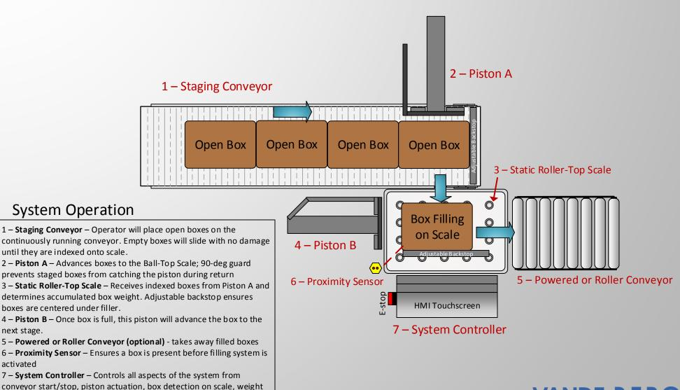
accumulation, signal transmission to filler and storage of all weights in SQL database. (System can be programmed to emit a pulse signal to
