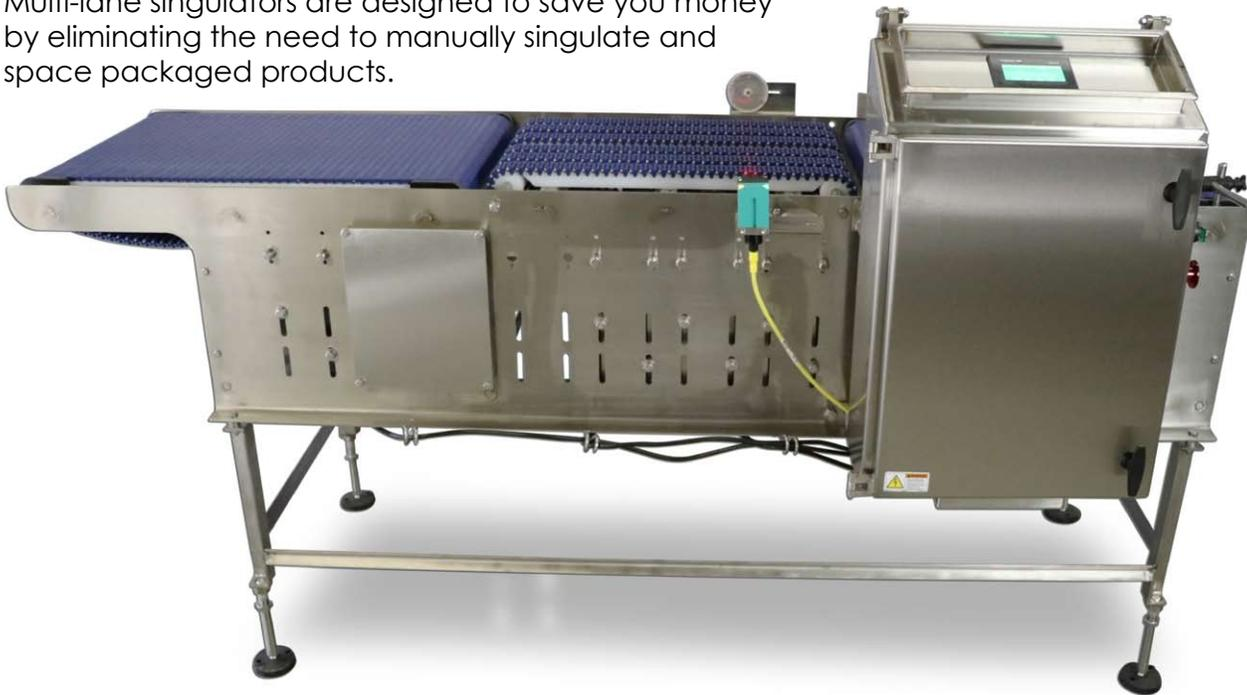
Multiple belt lanes permit one machine to accommodate varying product widths. This unit can singulate product widths spanning 2 or 3 belts. An added feature of this product is a cantilevered conveyor for an application such as protruding through a wall.
