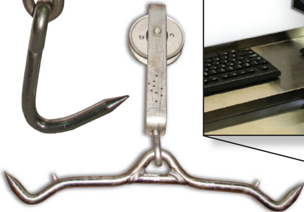
Carcass trolleys used for either beef or pork (pictured in order from left to right).
