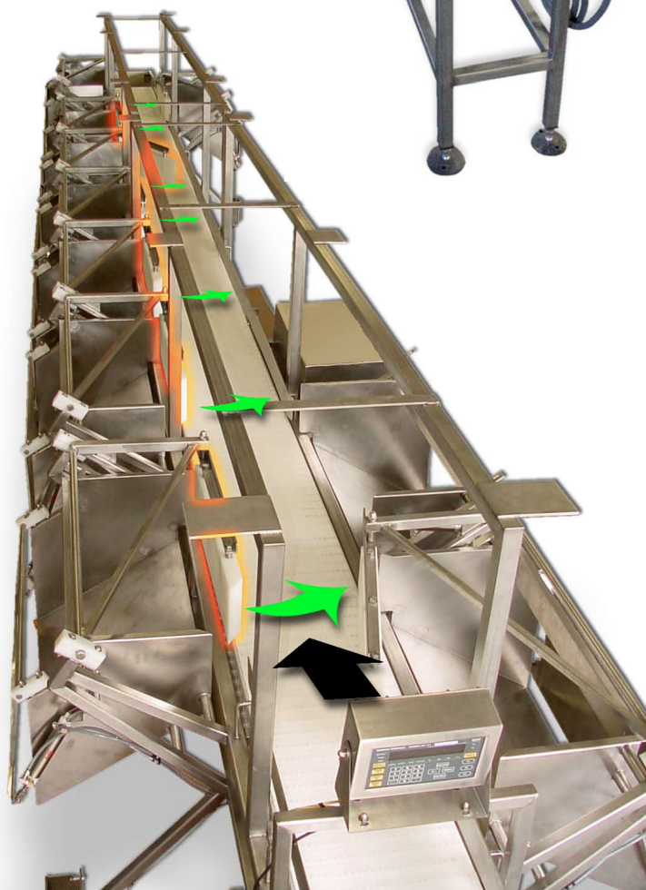
Whole hams were sorted based on weight, into various bins or combos via this conveyor sorting system
