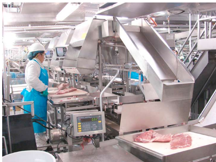
Rib sorting by weight and grade
