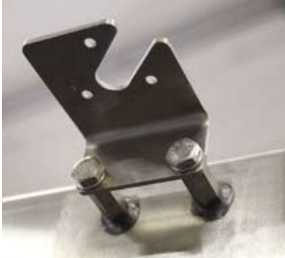
External flanges allow components (i.e. light bars, antennas) to be connected to the flange vs. securing the component directly to the enclosure, which would require drilling holes and creating a potential water entry point.
