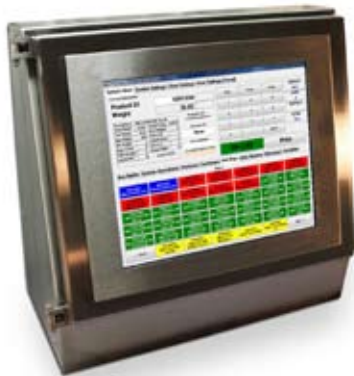
Touchscreen & embedded controller enclosure
