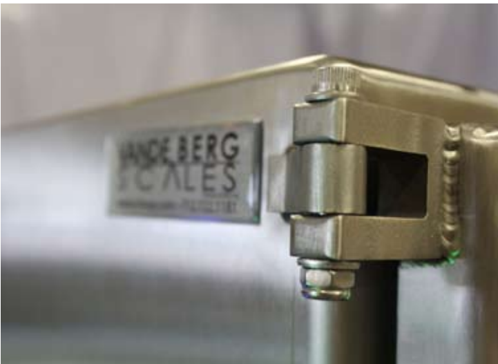
Double-shear point external hinges allow the door to make an even seal around the entire outside edge vs. internal hinges which often have reduced seal material in the vicinity of the hinge.
